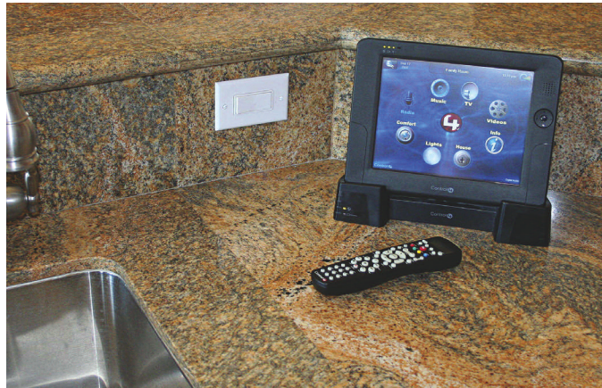
Controls such as this touchpad by Control4 allow users to set lighting, HVAC and security while they do the dishes.
